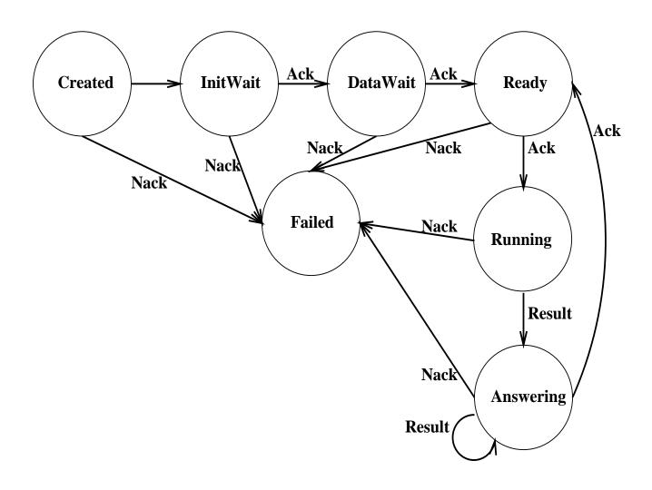
Figure 2: Process State Transitions
