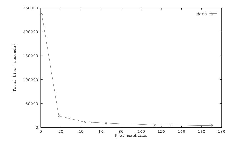
Figure 4: Results of Machines vs. Time to Render (excludes single machine run)
