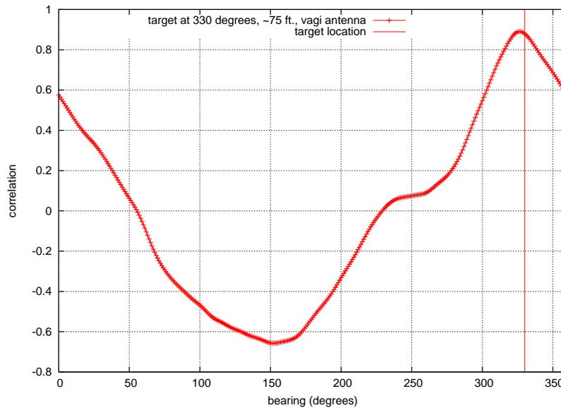
Figure 8: Correlation values of the June 16 Vagi antenna trials, with the first trial as training data and the second as testing; the maximum correlation occurs at  $326^\circ$ .
