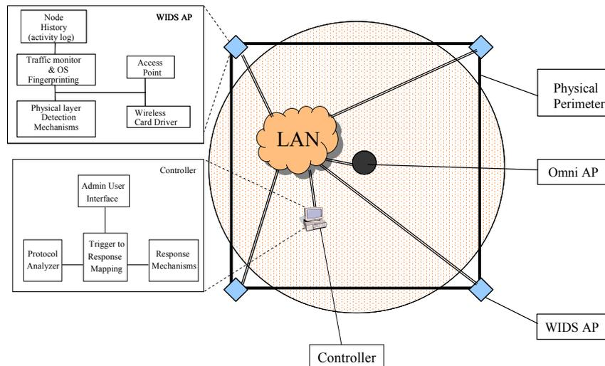
Figure 2: Intrusion Detection System Overview
