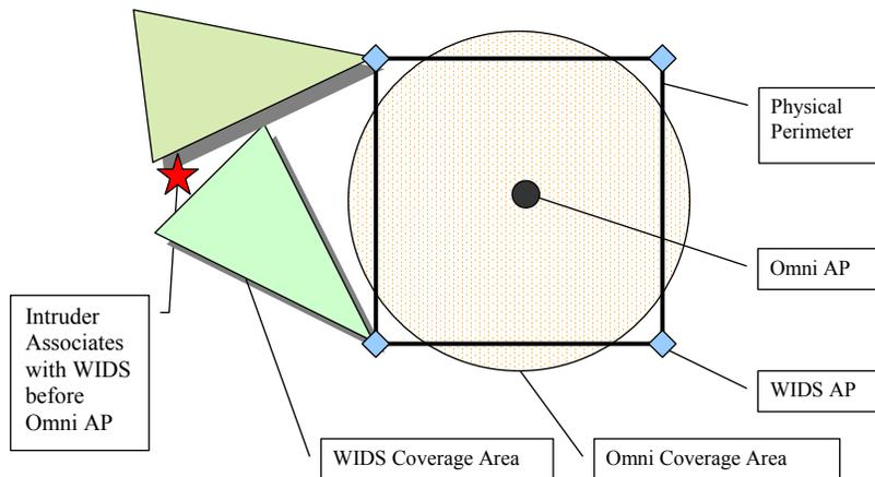
Figure 1: WIDS access point protecting a perimeter
