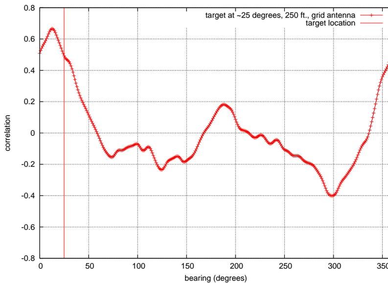
Figure 5: Correlation values of the May 9 grid antenna trial with the April 11 training data; the maximum correlation occurs at 13°.
